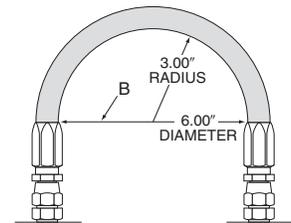
Maximum bend radius is measured on the inside bend of the hose. To determine minimum bend, divide the total distance between ends (B length) by 2. For example  $8 = 6$ , minimum bend radius = 3.
