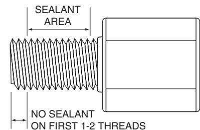
**Note:** If Teflon tape is used, it should be wrapped no more than  $1\frac{1}{2}$  to 2 turns in a clockwise direction when viewed from the thread end.
