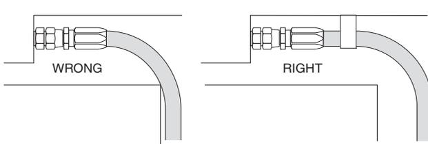
Install hose runs to avoid rubbing or abrasion. Use clamps to support long runs of hose or to keep hose away from moving parts. It is important that the clamps do not allow the hose to move. This movement will cause abrasion and premature hose failure.
