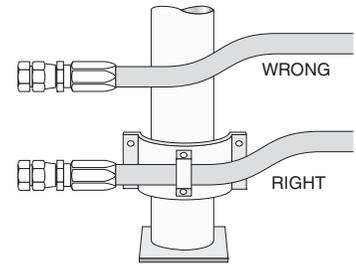
Keep hose away from hot parts. High ambient temperatures will shorten hose life. If you can not route it away from the heat source, insulate it.
