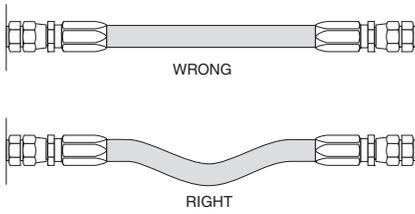
In straight hose installations allow enough slack in the hose line to provide for changes in length that will occur when pressure is applied. This change in length can be from +2% to -4%.
